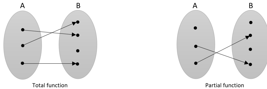
Figure 3.2.: An example of a total function (left) and a partial function (right)
