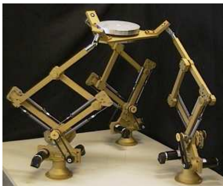
Figure 1.4: Spatial 6-DOF mechanism balanced using springs (Courtesy of Laval University)
