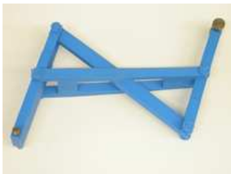
Figure 1.5: Dynamically balanced planar 4R, Gabriel's mechanism (courtesy of Laval University)
