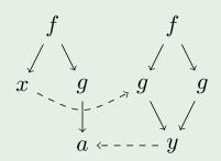
• With implicit application, the binding for a variable can be determined by traversing the graph depth first, left to right.
