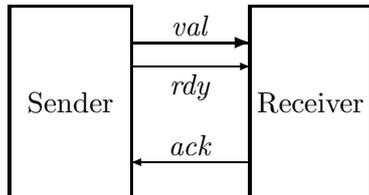
Data is sent on *val*, and the *rdy* and *ack* lines are used for synchronization. The sender must wait for an acknowledgement (an *Ack*) for one data item before it can send the next. The interface uses the standard two-phase handshake protocol, described by the following sample behavior.
