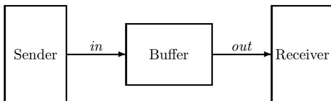
Values are sent over *in* and *out* using the asynchronous protocol specified by the *Channel* module of Figure 3. The system's specification will allow behaviors with four kinds of non-stuttering steps: *Send* and *Rcv* actions on both the *in* channel and the *out* channel.
