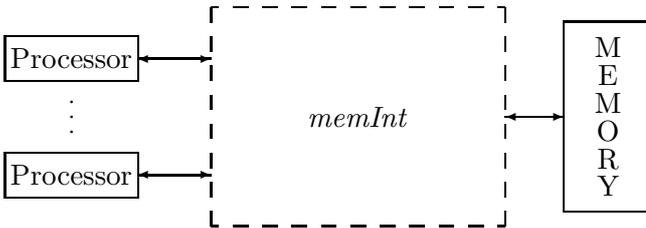
In this section we specify what the memory is supposed to do, then we specify a particular implementation of the memory using caches. We begin by specifying the memory interface, which is common to both specifications.
